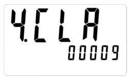
Press "key to clear data logger memory for last record and exit the mode.
